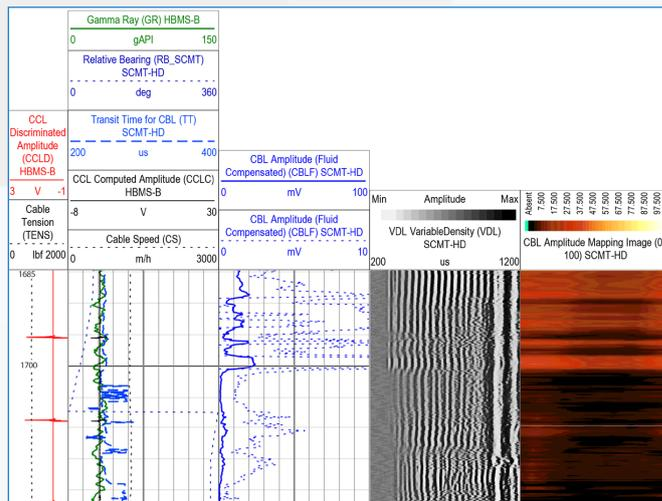
*In a Thailand field known to have annular pressure problems, wells cemented after conditioning with CemPRIME Scrub spacer experienced no such problems (from SPE-180624).*
