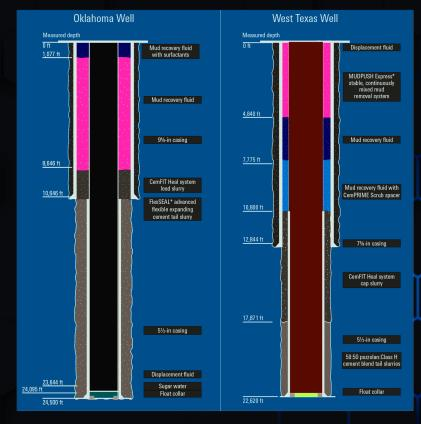
In Oklahoma, using a relatively small volume of CemFIT Heal system as a lead slurry cap maintained well economics while eliminating SCP. In Texas, the CemPRIME Scrub spacer system prepared the well for CemFIT Heal system lead slurry cap and pozzolan blend cement, also eliminating SCP.
