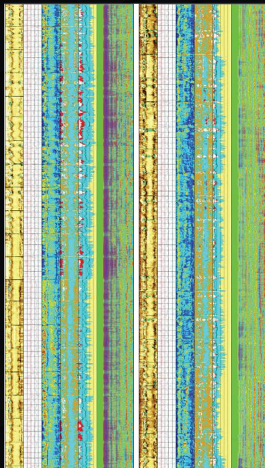
*In the conventionally cemented well, left, the cement bond is poor, and material in the channel is weak and uniform, which is common for drilling fluid. In the well cemented with Fulcrum technology, cement bond is improved, and the higher impedance with texture in places indicates a uniform substance with some mechanical strength.*
