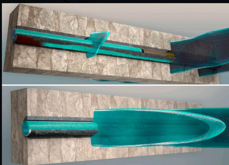
*Fulcrum technology improves fracturing performance by reacting with NAF to limit its mobility and improve resistance to out-of-zone fracturing fluid flow. Top, fracturing fluid migrates between stages behind the casing through mud channels, resulting in stunted fracture extension. Bottom, Fulcrum technology reduces mud channel permeability and mobility, keep the fracturing fluid in the intended stage to improve fracture length and efficiency.*
