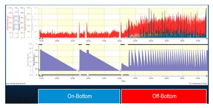
The figure below displays an example of external Bias unit damage which occurs during an extended off-bottom cleanup cycle.
